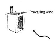
If the pit extends to the side of the superstructure the vent pipe should also face the prevailing wind.
