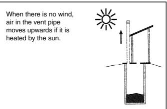
The upward movement of air in the vent pipe reduces nuisance from smells and insects.
