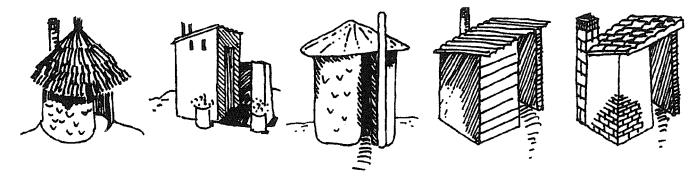
Ventilation is provided in VIP's by a vent pipe with flyproof netting at the top.
